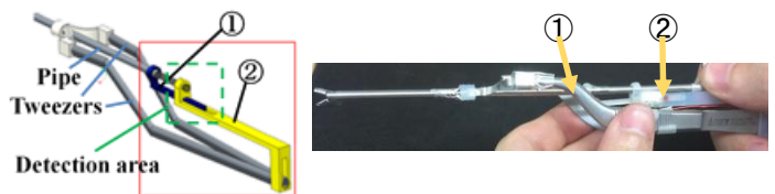
Fig.4 Tip open-close detect mechanism
